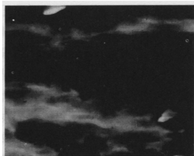
Fig. 2 TEM of the axial section of monofilament with 20% polyaniline content ( \times 1 \times 10^4 )
